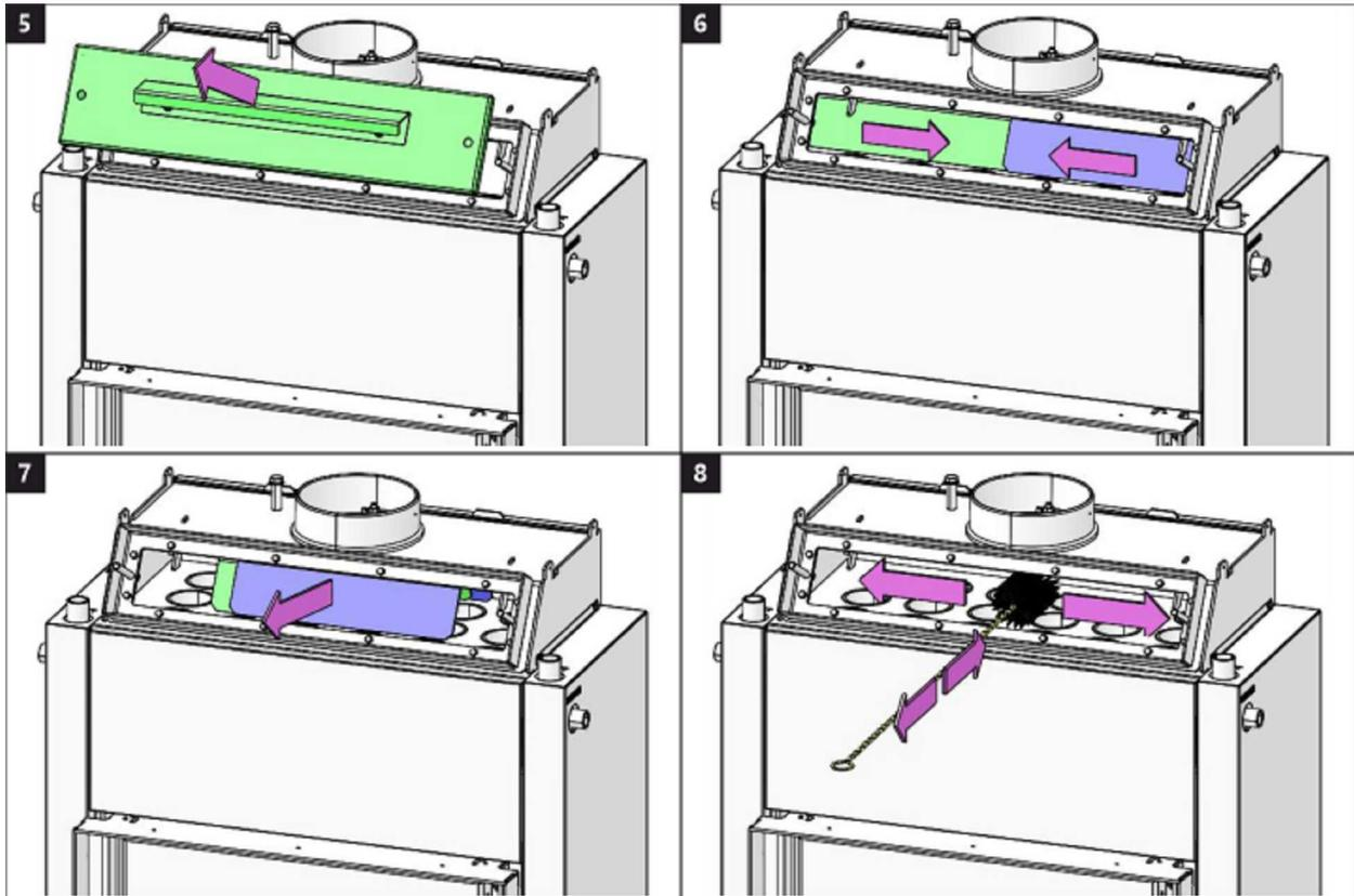
Cleaning of flue gas path 3 | Reinigung Rauchgaswege 3
